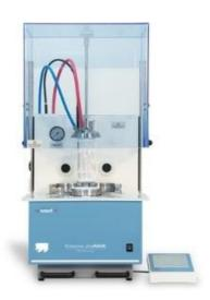
Milestone UltraWAVE ECR with internal temperature and pressure control in all vessels, 660 terminal with easyCONTROL software installed.
