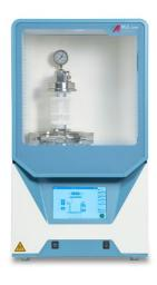
Milestone ultraWAVE 3 with internal temperature and pressure control in all vessels, built-in touchsceen with easyCONTROL software installed.
